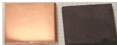
Fig. 9. Copper samples before and after \text{RuO}_4(\text{g}) treatment.
