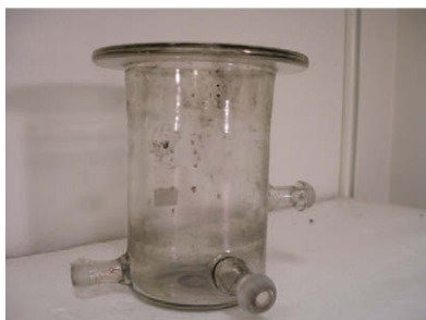
Fig. 1. The reaction vessel after the completed experiments. Observe the black spots of ruthenium deposits.
