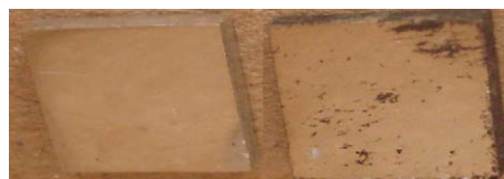
Fig. 8. Aluminium samples before and after \text{RuO}_4(\text{g}) treatment.
